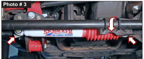
assembly stud mount. Secure, but Do Not Completely Tighten.
