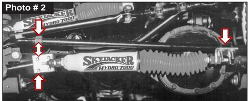
3. Extend Skyjacker Bracket \ Shaft End exactly half way (4-1/4 Inches).
