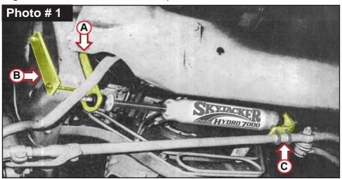
3. Position Skyjacker # 83037 Tie Rod Bracket 'C' against top of tie rod toward inner tie rod connection. Install supplied 5/16" x 1-1/4" x 1-3/4" U-Bolts from bottom-to-top around OEM tie rod through Skyjacker bracket mounting holes.
