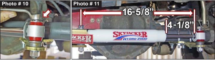
Note: Tighten Center Axle Bracket Assembly so there is 1/4-Inch clearance between Skyjacker steering stabilizer bodies & upper OEM drag link assembly.
