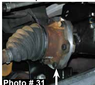
Passenger side shown with one 15/16" cv-spacer.
