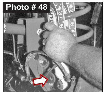
37. Install Skyjacker # DBE20 Front Brake Line Relocation Brackets. Skyjacker bracket has a short 90° bend at bottom. Position 90° bend facing forward & align with OEM brake line bracket axle mount. Attach with OEM bolt using a 13mm socket \ wrench. (Photo # 49)
