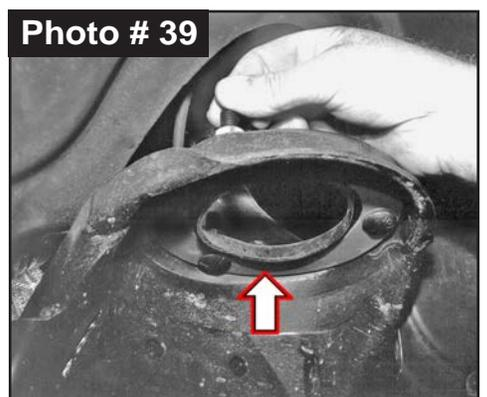
**Note:** Skyjacker **D50** Front Coil Springs Are Side Specific & Must Be Installed on Appropriate Side: Part Number Is Paint Stamped on Each Coil Spring & Labeled Driver or Passenger. 1/2 Ton & Light 3/4 Ton Vehicle *WITHOUT* V10\Cummins Engine.
