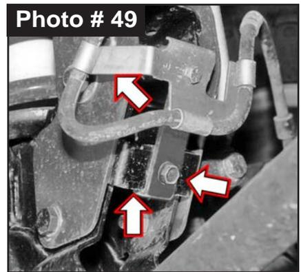
Attach OEM brake line bracket to Skyjacker Bracket with supplied 1/4" x 1" Fine thread Bolt & 1/4 Nylon Insert Lock Nut using a 7/16" socket \ wrench. **Tech Note:** It may be necessary to bend OEM bracket side wing out for clearance on Skyjacker Upper Link Bracket bolt head. **NOTE:** On 2001-2002 2500 \ 3500 Models with Cummins Diesel, Driver Side metal brake line Will Need to be bent out & away slightly for clearance between the Dual Shock & OEM Shock Bracket.
