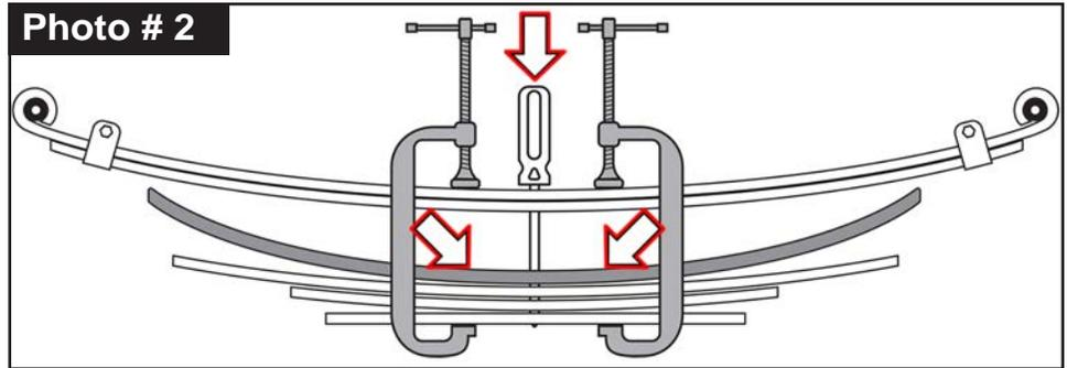
**CAUTION: Do Not Use Skyjacker Tie Bolts to Draw OEM Leaf Springs Together. Failure of Any Component Can Cause an Explosive Disassembly & Possible Injury!**
