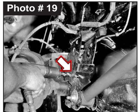
**Note:** Skyjacker Upper Link Brackets Are Side Specific & Must Be Installed on Appropriate Side: # DULRB-L \ DULRB-L2K Driver Side & # DULRB-R \ DULRB-R2K Passenger Side.
