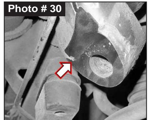
Rotate Track Bar Bracket so that brace is flat against crossmember. If clearance is needed for brace, mark & grind with die grinder or file until clearance is obtained, then position brace flat against crossmember. (Photo # 32 & # 33)
