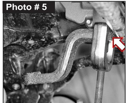
9. Mark position of OEM pitman arm on steering gear box sector shaft. Transfer an index mark over to Skyjacker pitman arm.
