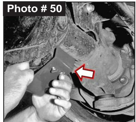
**Tech Note:** Be sure each carriage bolt aligns & locks into square holes of Skyjacker Skid Plate.
