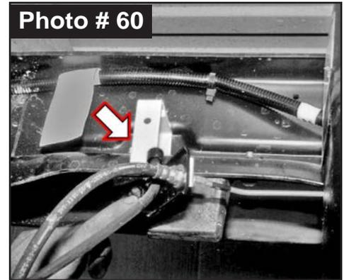
Attach OEM brake line bracket to Skyjacker Bracket with supplied 1/4" x 1" Fine thread Bolt & 1/4" Nylon Insert Lock Nut using a 7/16" socket \ wrench. **Tech Note:** Carefully reform OEM brake line to gain slack needed to bolt OEM brake line harness bracket to Skyjacker bracket.
