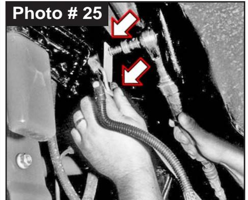
23. Unplug electrical line at vacuum actuator valve & release plastic OEM retaining clip at bracket. Reconnect electrical line to actuator valve.
