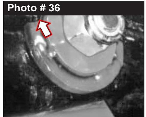
28. Remove supplied 18mm Nylon Lock Nut from OEM frame mount & Skyjacker bracket using 27mm socket \ wrench.
