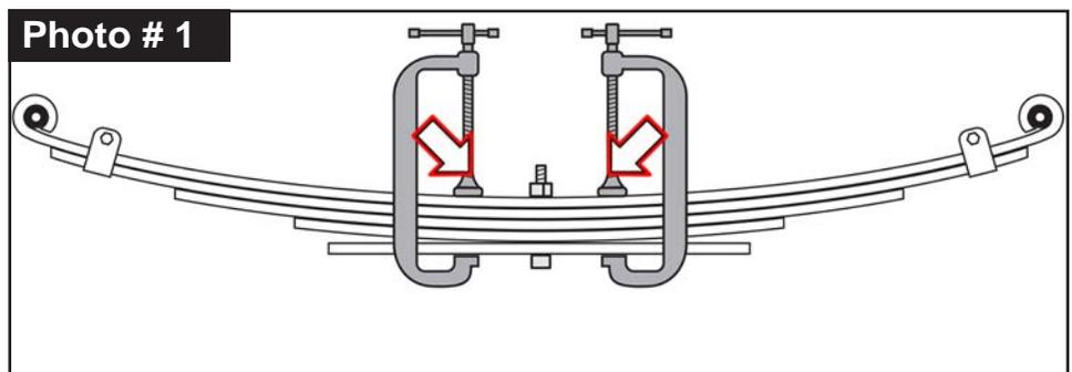
9. Carefully & slowly loosen C-clamps equally on each side until leaf spring expands completely. Remove C-clamps.
