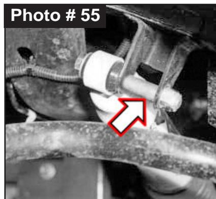
Insert supplied 1/2" x 4" Bolt with 1/2" SAE Washer through cylinder eye of stabilizer & outer mounting tab. Place supplied 1.50" Steel Sleeve inside mounting tabs. Attach with supplied 1/2" Nylon Insert Lock Nut using a 3/4" socket \ wrench.
