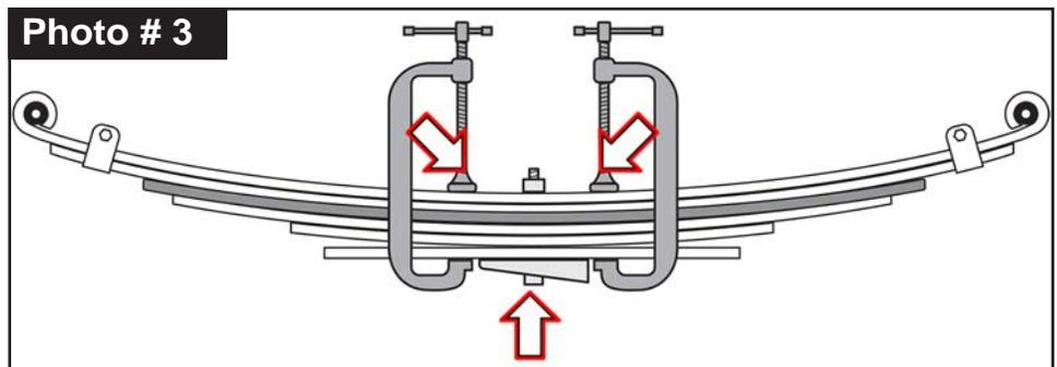
**Torque Specifications:** 3/8" Tie Bolt = 17 ft lbs. \ 204 in lbs. 1/2" Tie Bolt = 41 ft lbs.
