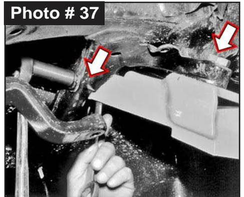
29. At crossmember, move OEM brake line clamp over \ down approximately 2-inches.
