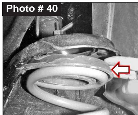
**WARNING:** On Dodge Ram trucks, SKYJACKER® replacement front shock absorbers limit extended position of the front suspension! The use of shocks other than those supplied, may cause coil disengagement, adverse steering angles, brake line failure, driveline component failure and/or other related component failure! The use of other shocks will void your SKYJACKER® Warranty!
