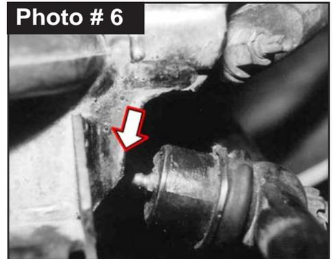
Front shock absorber upper OEM mount using a 5/8" socket \ wrench. Torque 35 ft-lbs.
