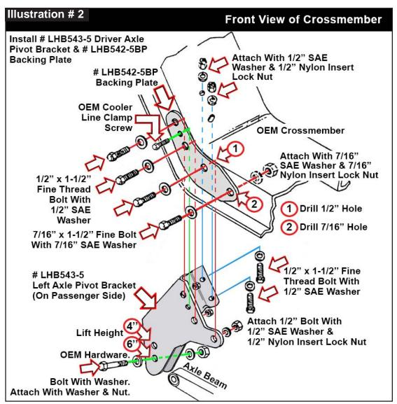
Use a wire brush, grinder brush or similar tool to remove any undercoating. Skyjacker bracket must be installed on a smooth & clean surface. Then paint all exposed metal.
