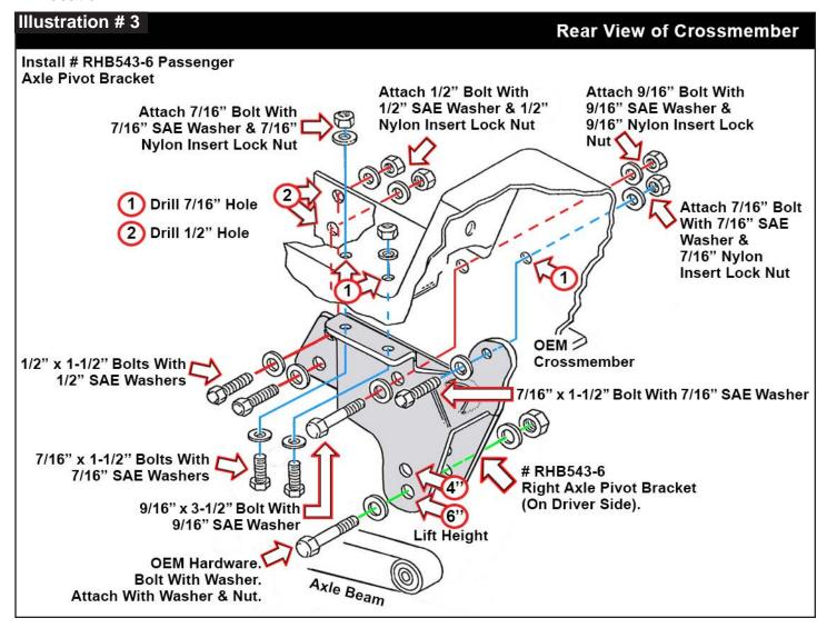
Use Skyjacker bracket as a guide for a total of five (5) mounting holes on OEM crossmember. Two (2) 1/2" mounting holes & three (3) 7/16" mounting holes.
