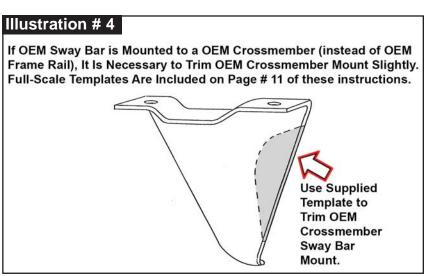
Remove OEM crossmember from OEM sway bar mount. Trim crossmember using a power grinder or cut-off tool. **Note:** File smooth any burrs or sharp edges, then paint or undercoat all exposed metal surface areas.
