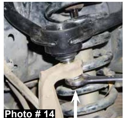
25. Grease each new Skyjacker upper A-arm ball joint using a grease gun.
