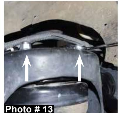
22. Install each OEM lower strut mount to each OEM lower A-arm using the OEM hardware & a 1 1/16" & 1 3/16" socket / wrench for 2009 - 2013 models or a 19mm socket / wrench for 2014 - 2020 models.
