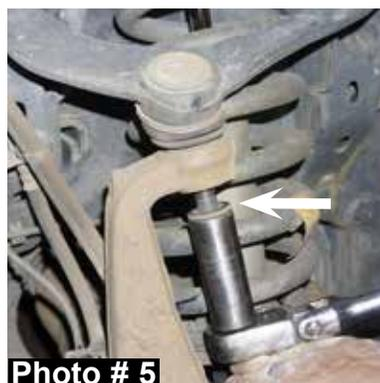
11. Remove the OEM upper strut retaining nuts from each OEM strut assembly using a 15mm socket / wrench & remove each OEM strut assembly. (See Photo # 6)
