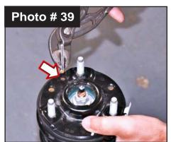
7. Remove alignment roll pin from top of OEM strut assembly using pliers or vise grips. (See Photo # 39)
