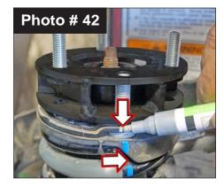
9. Move around strut assembly (approximately 1/4 turn) & mark alignment of first hole\stud in Skyjacker Spacer with top hat upper strut mounting isolator & rubber isolator at top of OEM strut. (See Photo # 43) Remove Skyjacker Spacer.
