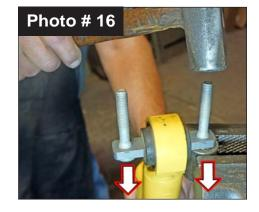
21. **Note:** For proper reassembly realignment, mark top hat upper strut mounting isolator, rubber isolator & coil spring at top of strut.
