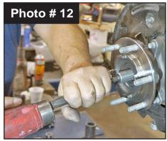
16. Ease knuckle to rest back away from front strut. **CAUTION**: Do not let knuckle fall to side abruptly. It could cause damage to brake lines or pull CV axle shaft out.
