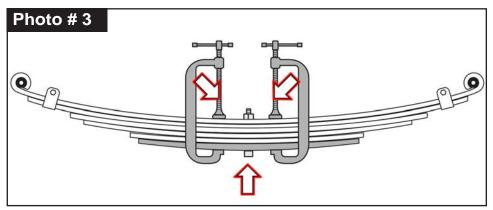
11. Once C-clamps have drawn leaves securely together, use locking pliers to hold tie bolt head & tighten tie bolt nut with a wrench. <u>Caution</u>: Do not use an air gun to tighten tie bolt. An air gun could strip or over torque \stretch tie bolt.
