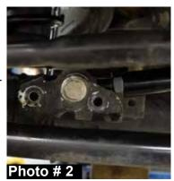
8. Tighten the jam nut of the new Skyjacker rod end using an adjustable wrench.
