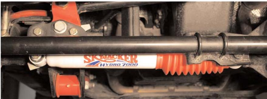
10. Install new Front Skyjacker shocks using hardware supplied. Install tires/wheels.
