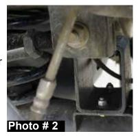
8. Tighten the jam nut of the new Skyjacker rod end using an adjustable wrench.
