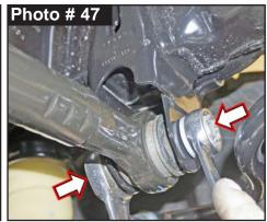
6. <u>Rubicon Models</u>: OEM rear locker must be disconnected so wiring connectors are not over-extended. On rear axle, unplug locker wiring harness from side of center differential housing. <u>Tech Note</u>: Safety lock clip must be slid rearward to unlock. Press & hold rearward tang down, grab connector & pull away while from plug-in.
