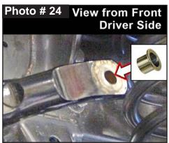
24. Install Skyjacker Sway Bar End Link Assembly upper eye mount with supplied 12mm x 70mm Bolt with a 7/16" USS Washer from inside-to-outside through sway bar.
