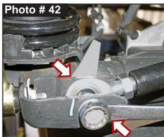
37. <u>Adjust\Align Track Bar</u>: Check front of vehicle to make sure body is centered over front tires\wheels. Using a measuring tape, measure from inside of tire to frame on driver side, then measure passenger side.
