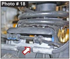
using a 7/32" hex key socket\wrench & 9/16" socket\wrench. Torque 25 ft-lbs.
