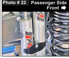
hex head bolts using a hex key socket (one (1) front & one (1) back). Position clamp into place around shock body & reservoir cylinder. Secure, but **Do Not Completely Tighten**.
