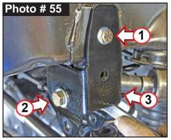
13. Second, insert one (1) supplied 9/16" x 1-1/4" Fine Thread Bolt with 9/16" SAE Washer through bracket \ OEM track bar mounting holes from rear-to-front. (Photo # 55) Attach with 9/16" SAE Washer & 9/16" Nylon Insert Lock Nut on inside using a 13/16" & 7/8" socket \ wrench.
