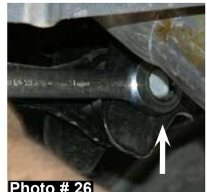
10. Remove the OEM rear bump stops & install the new Skyjacker rear bump stop spacers between the frame & the OEM rear bump stops using the supplied 10mm x 80mm bolts & washers. (See Photo # 27)
