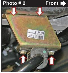
6. Attach OEM sway bar frame mount with two (2) supplied 7/16" x 1-1/2 Fine Thread Bolts with 7/16" SAE Washers up from bottom-to-top. Attach with 7/16" SAE Washer & 7/16" Nylon Insert Lock Nut using a 5/8" socket\wrench.
