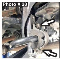
Connect OEM sway bar mounting bracket to Skyjacker bracket using OEM bolts & a 12mm socket\wrench. (See Photos # 28) Torque to 25 ft.\lb.
