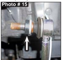
18. Jounce vehicle a couple of times. This will help suspension settle to new ride height. Torque Skyjacker \ OEM strut upper mount using a 15mm socket \ wrench to 30 ft.\ lb. Torque both OEM sway bar end links to Skyjacker Sway Bar End Link Bracket to 45 ft.\ lb.
