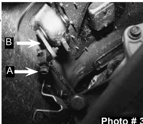
5. On 5 speed models, engage the clutch & check the transmission shifter to see if it will go into 2nd gear. If not, the shifter housing on the floor will need trimming. Remove the center console, pull back the carpet, remove the screws holding the shifter boot to the floor, & trim or grind the floor board until sufficient clearance is obtained. (See Arrow in Photo # 4) Shift through each gear to check clearance at this time. Now reinstall the shifter boot, carpet, & console.
