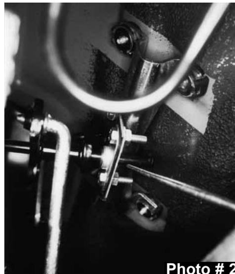
3. Check to make sure that the transfer case will fully engage at each end of the shifter travel. If linkage adjustment is required, see Step # 4.
