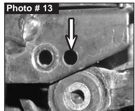
24. Locate Skyjacker # SBE401-L Front Sway Bar End Links. Coat # ES25 1.50 Long Steel Sleeves with a water resistant grease & press into upper & lower end links mounts.
