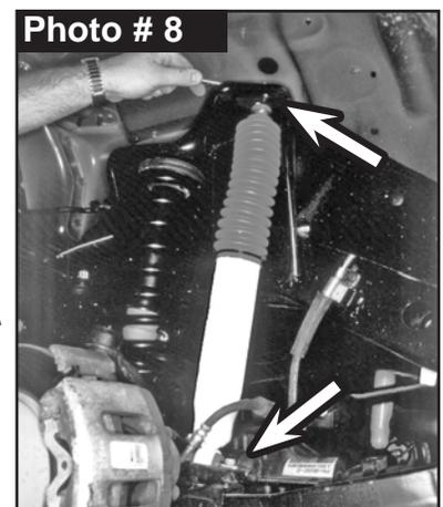
18. Install Skyjacker ADX front shock. **Tech Note:** ADX Remote Reservoir are to be mounted with the remote reservoir toward rear for proper clearance (opposite side of coil spring mount). (See Photo # 9 & # 10)
