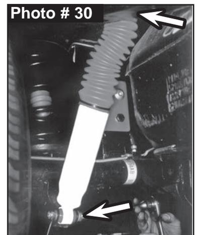
Install Skyjacker ADX rear shock. Connect upper bar pin mount with OEM hardware using a 15mm socket \wrench.
