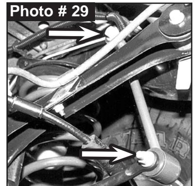
13. Coat with a water resistant grease & press # 142118 Steel Sleeves into upper & lower mounts of Skyjacker # SBE500-L Rear Sway Bar End Links.
