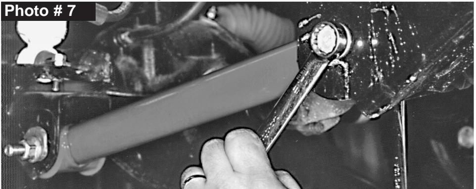
16. Install Skyjacker front coil springs. Insert coil spring into upper tower first. Be sure that the coil & OEM spring isolator are indexed to seat properly, then raise axle enough to hold coil spring in place. Re-install OEM bottom clip & bolt to driver side OEM coil spring using a 13mm socket \wrench. Torque 20 ft.-lbs.
