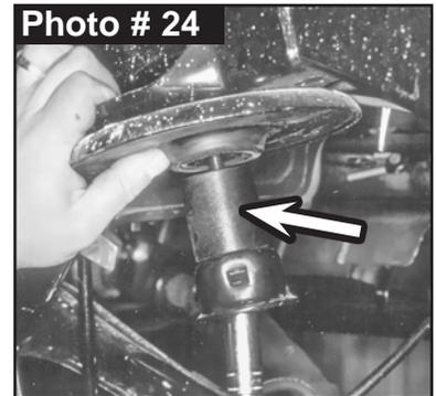
9. Install Skyjacker # TJRTB-B Rear Lower Track Bar Bracket over OEM rear lower track bar bracket at axle.
