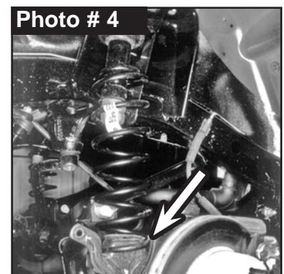
13. Remove the OEM 10mm bolt from inside the OEM bump stop cup using a 15mm socket \wrench.
