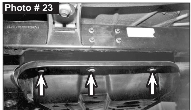
Apply a few drops of supplied # LT100 Thread Lock Compound onto supplied 12mm x 80mm Metric Bolts. Install with 1/2 SAE Washer on bolt & tighten using a 18mm socket \ wrench. (See Photo # 23) Secure, but **Do Not Completely Tighten** until all six (6) are installed. Torque 75 ft-lbs.
