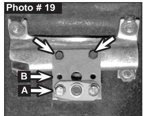
28. Connect OEM shifter linkage ball swivel bracket to Skyjacker bracket in lower mounting holes. Connect with supplied 1/4" x 1" Bolts with 1/4" SAE Washers & attach with 1/4" Nylon Insert Lock Nut using a 7/16" socket \ wrench. (See Photo # 20)
