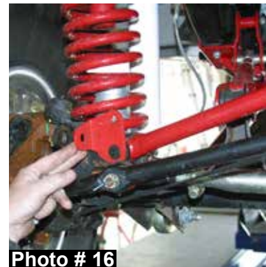
5/16" x 3/4" thread cutter flange bolt.
